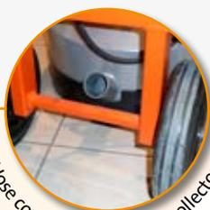
Hose connector to fit dust collector.
