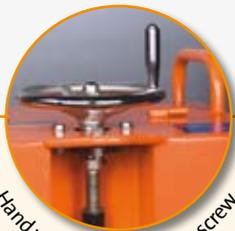
Hand wheel with endless screw depth control system.
