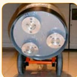
3 planetary 155 mm diameter rotating heads.
