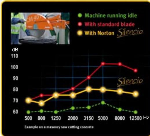
Two complementary dampening technologies make the NORTON SILENCIO especially efficient in reducing the high-frequency noise, with reduction of the total noise level by up to 15 dB(A), and up to 25 dB(A) in some frequency ranges.
