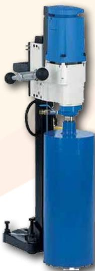
Comprising of Shibuya R1721 110V 3.0kW motor with 2 speed gear box and an RPM range of 450/900. It has a standard 1½” UNC motor spindle and is supplied with a Shibuya TS252 drill stand with swivel base and has a column height of 800mm.
