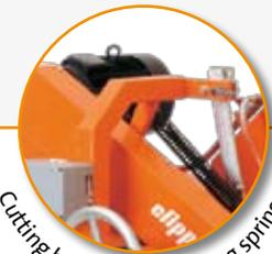
Cutting head with balancing spring.
