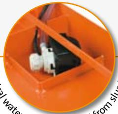
Electrical water pump protected from slurries.
