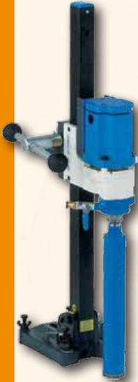
Comprising of Shibuya R1011 single speed 650RPM, 1kW drill motor, with standard 1½" UNC motor spindle.
