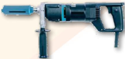
1.3kW single speed motor at 2,000 rpm for dry drilling up to 152mm diameter, fitted with centrifugal safety clutch.
