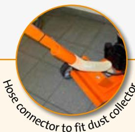
Hose connector to fit dust collector.
