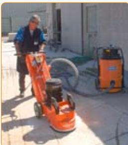
Use the machine with CV324 dust collector, for a dust free, healthy and comfortable working environment.
