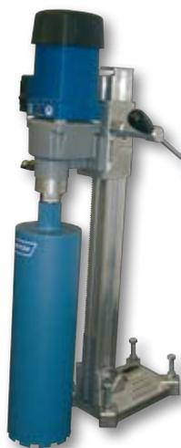
Single speed 420 RPM 2kW slow start drill motor, with standard 1½” UNC male, ½” BSP female motor spindle.
